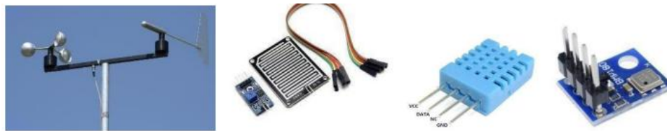
Fig. 2. Anemometer, Rain Detector, DHT11, and BMP180
